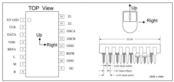
Figure 3-1a OM35APS Pin Configuration (Top View)
