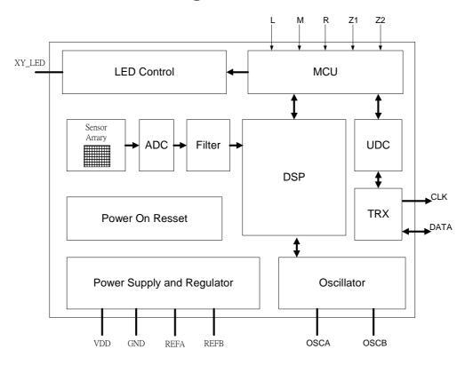
Figure 4-1 OM35APS Functional Block Diagram
