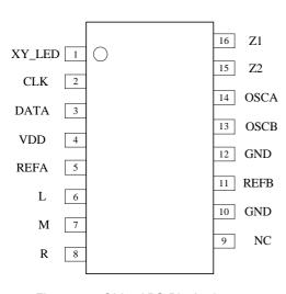
Figure 5-1 OM35APS Pin Assignments
