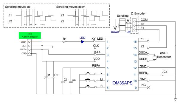
Figure 8-1 MODE-I for Basic Circuit
