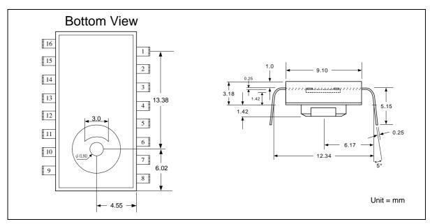
Figure 3-1b OM35APS Pin Configuration (Bottom View)
