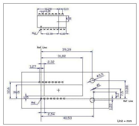
Figure 10-1 PCB Vias Layout for OM35APS
